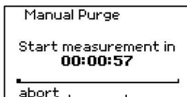
After purging the device independently returns again to the normal operation.
